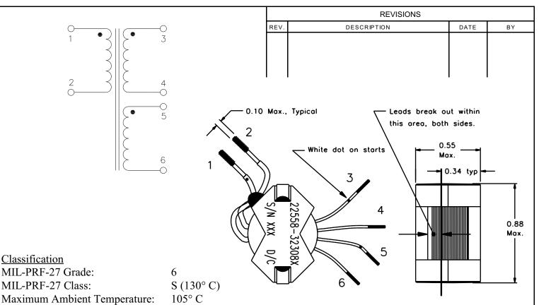
The absolute position of the connections is defined on Sheet 2.
